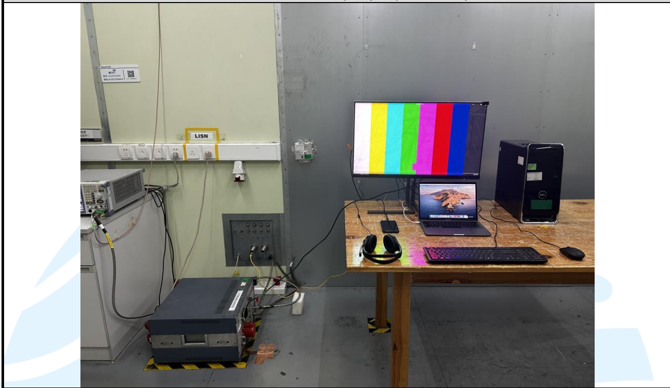
Conducted Emission (AC port) Test Setup
