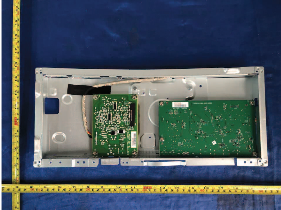
Figure 23. Internal view of enclosure for DC converter board
