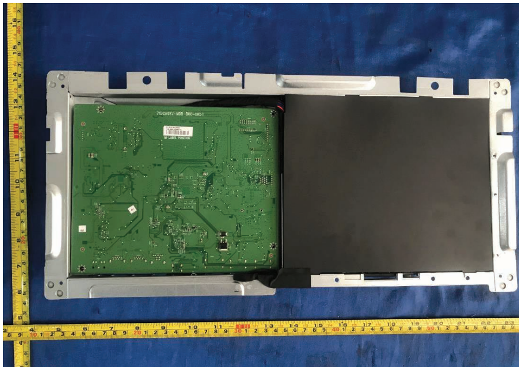
Figure 52. Internal view of metal enclosure
