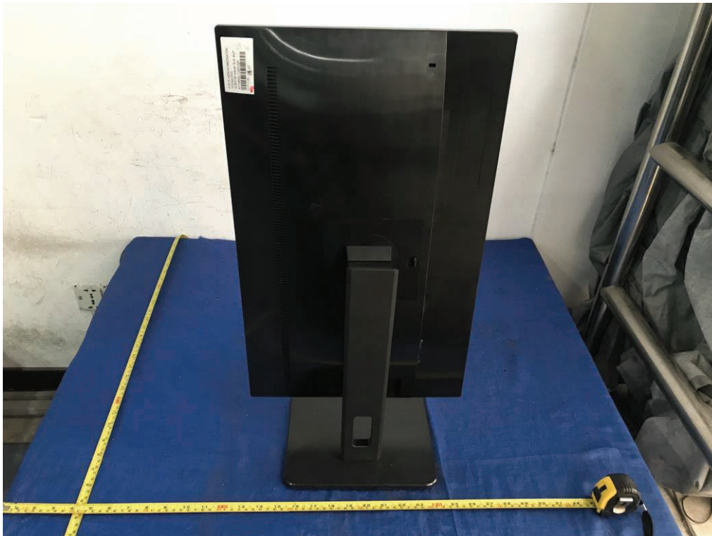
Figure 18. Rear view with plastic enclosure type B and base type B (vertical position)
