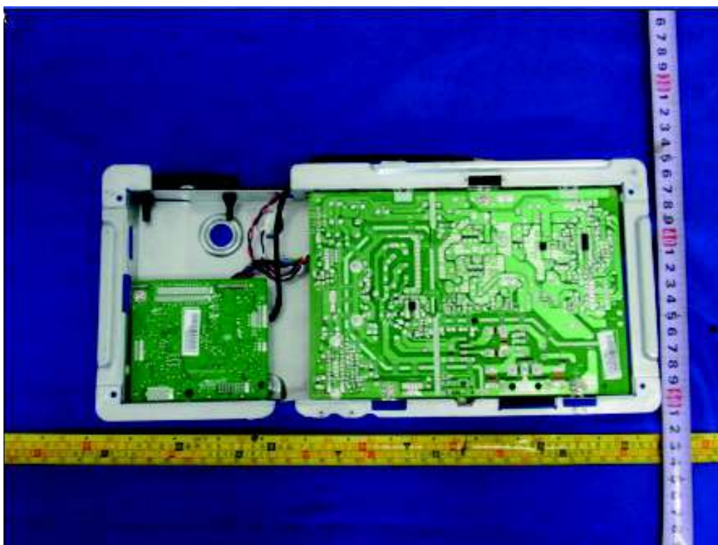
Figure 34. Internal view of metal enclosure type A without mylar sheet
