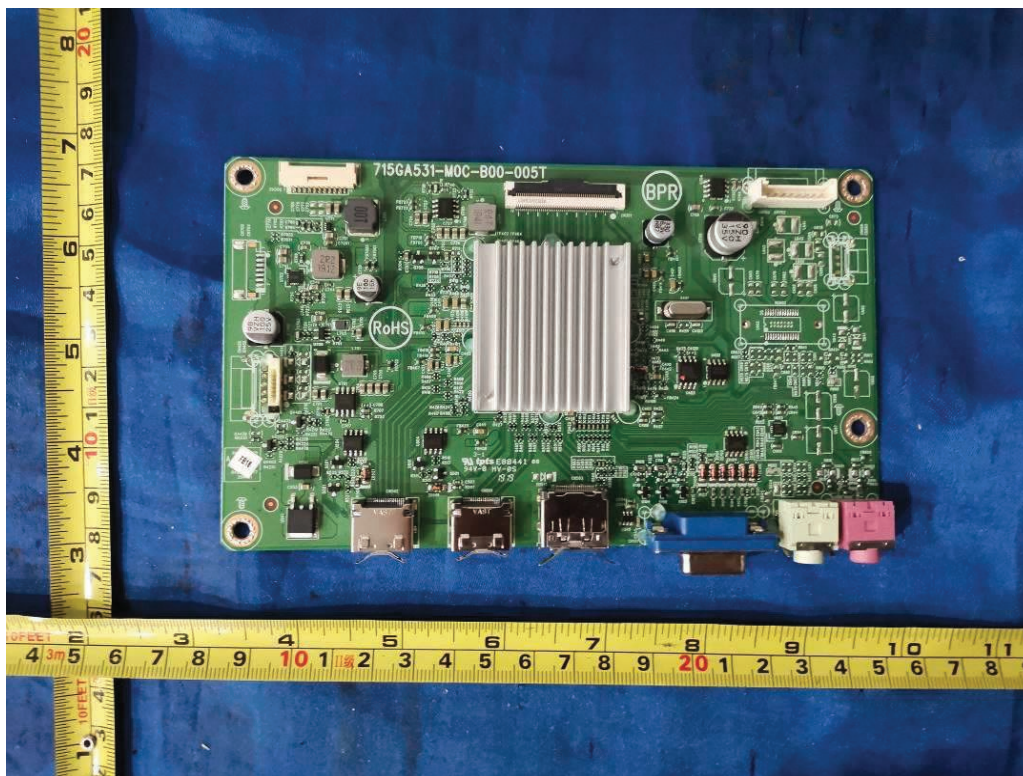
Figure 32. Main board 715GA531 used for 27.0 inch models
