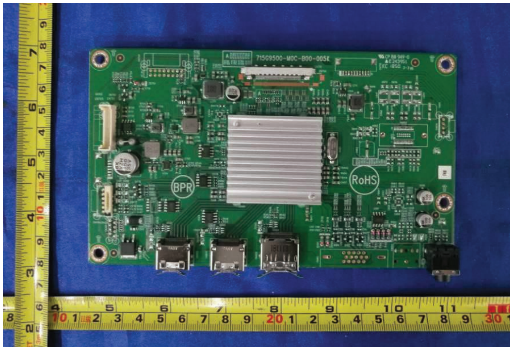
Figure 30. Main board 715G9500 used for 27.0 inch models
