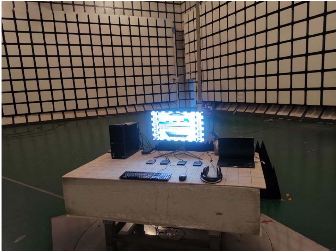
In 10m Anechoic Chamber Test 1GHz – 6GHz
