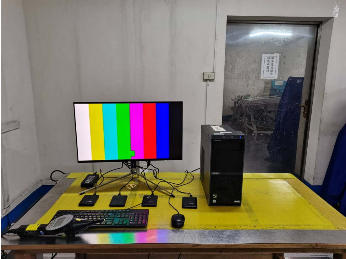
15.5. Photo of RF Strength Susceptibility Test
