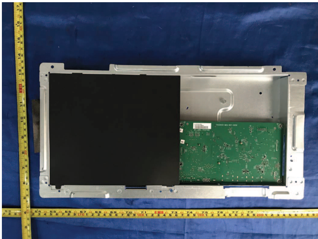
Figure 56. Internal view of metal enclosure Type C
