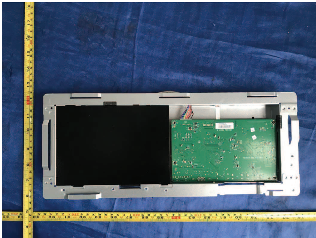
Figure 40. Internal view of metal enclosure Type B
