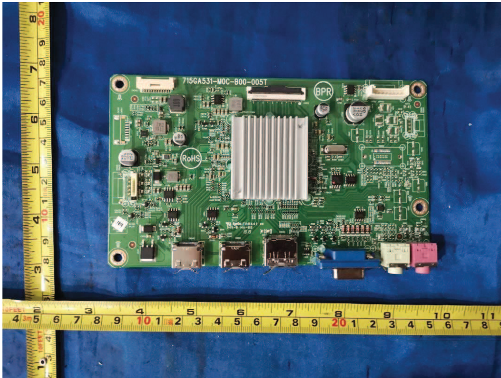
Figure 31. Main board 715GA531 used for 27.0 inch models
