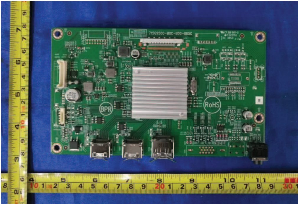
Figure 29. Main board 715G9500 used for 27.0 inch models
