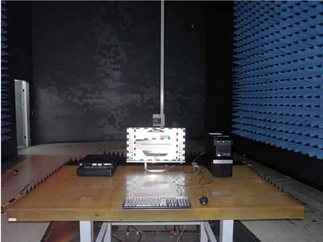
Front View of Radiated Measurement
